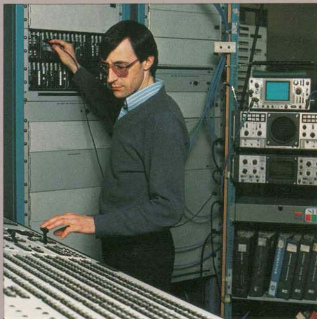
FINAL CALIBRATION AND SYSTEM TEST OF THE SERIES 80 SWITCHER
