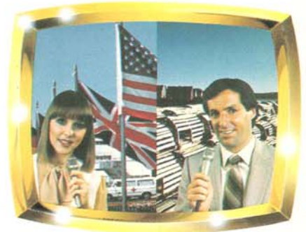
Figure 3 Wipe from a Chroma Key over one Background to another Chroma Key over another Background.
